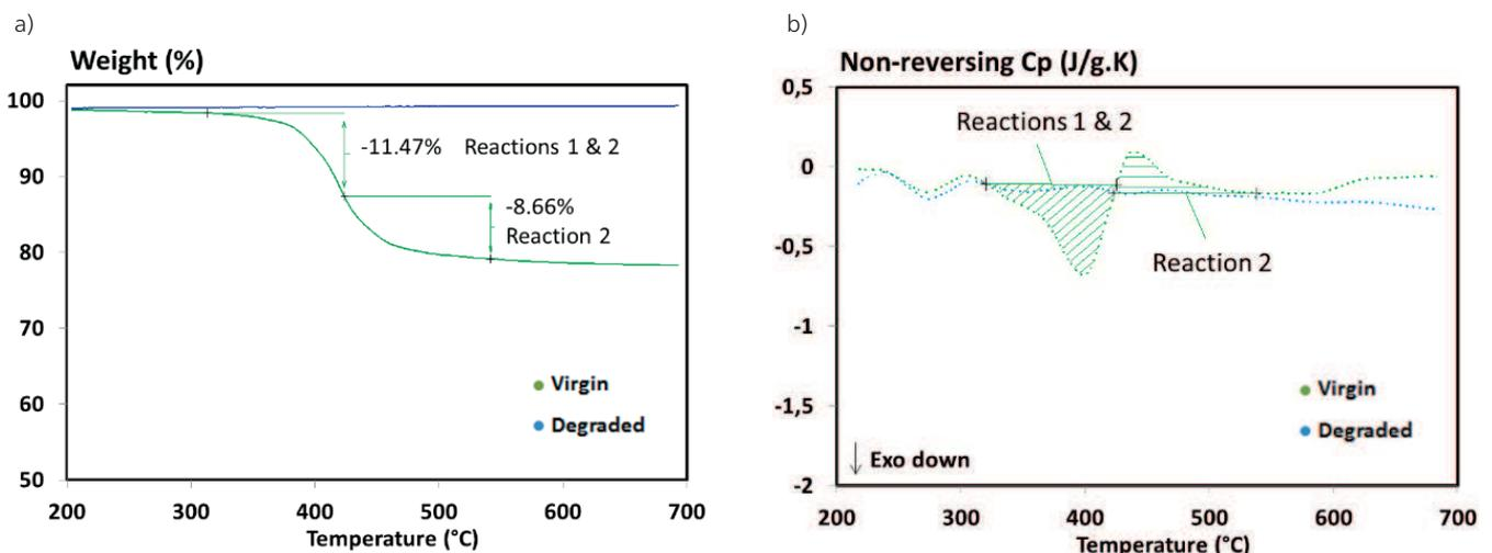
Figure 1. (a) Remaining mass and; (b) non-reversing specific heat capacity obtained during an STA test carried out under nitrogen to determine the heats of decomposition of T700/M21 [1]
