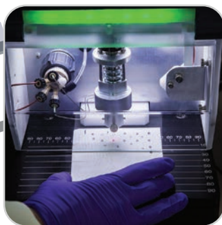
Plate Express ™ : TLC/CMS Mass Analysis of TLC spots
