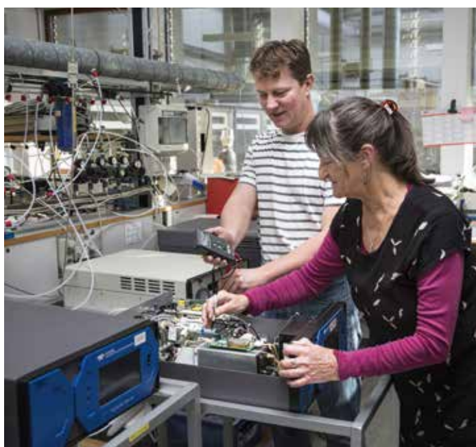
Reparation af NO x -monitor i DCE's akkrediterede monitorlaboratorium.
